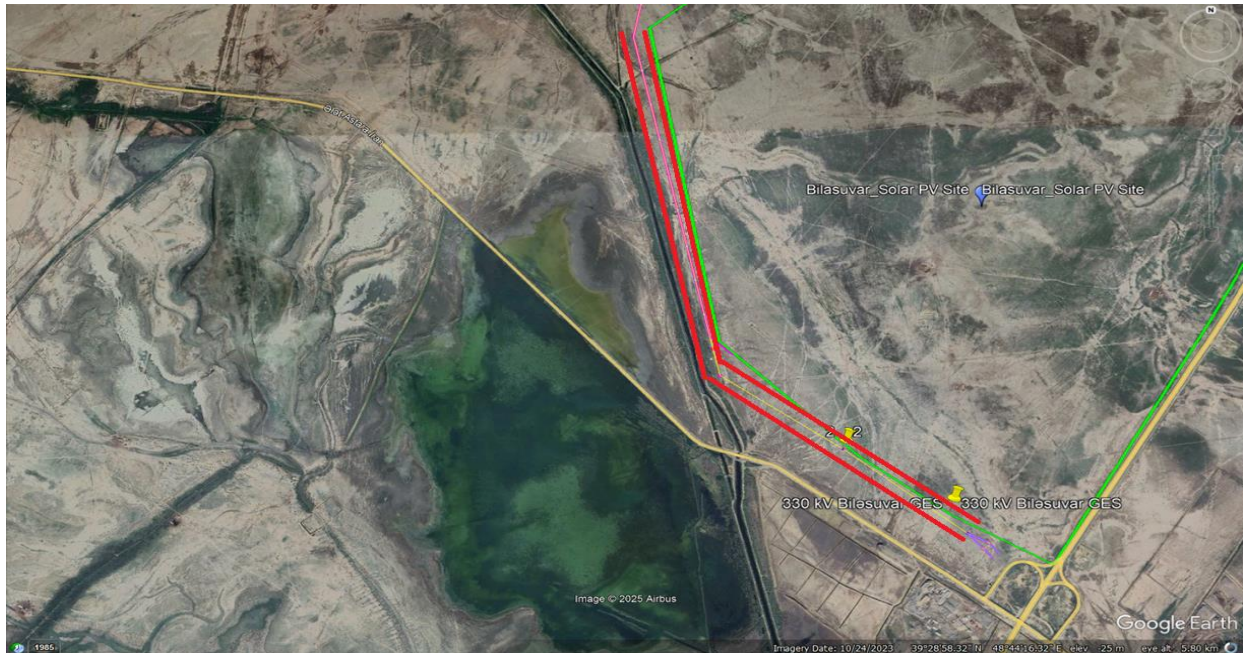
Figure 4. Bilasuvar SPP - Navahi SS bird flight diverters installation section (red lines)
